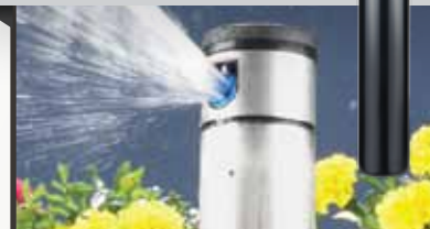
I-20-12: Overall height: 43 cm Pop-up height: 30 cm Exposed diameter: 4.5 cm Inlet size: 3/4" female
